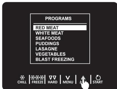
Recipes are preset ready-to-use programs that offer a series of cycles optimized by type of dish. When P3 is set to 0, any recipes that call for a setpoint for the needle probe are not displayed. The recipes can be modified before starting the cycle, but cannot be saved or over-written.
