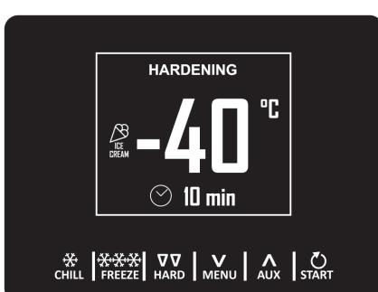
Access the SPECIAL CYCLES menu using the "AUX" key and select ICE CREAM HARDENING.
