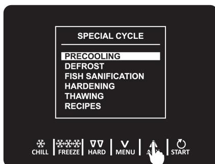
This is a refrigeration cycle of infinite duration that can precede all the operating cycles. It can also be used as a refrigeration cycle of infinite duration.
