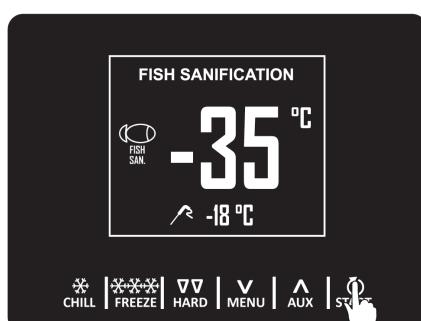
Access the SPECIAL CYCLES menu using the "AUX" key and select FISH SANITATION.
