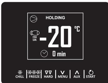
During a sanitation cycle, the device will always display the cabinet temperature and, depending on the phase in progress, the blast chilling end temperature or the duration of the holding phase.
