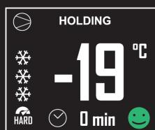
On completion of the blast chilling/blast freezing cycle, when the needle probe has reached the right temperature or the time period is finished, the buzzer sounds and the conservation phase begins. If the temperature controlled cycle is not completed in the allotted time, the problem will be notified by displaying an alarm message.
