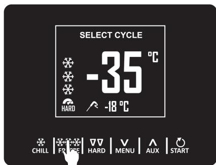
The blast chilling functions can be accessed quickly by pressing the key "CHILL".
