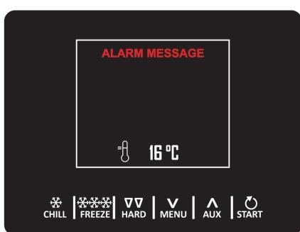
The alarms will be displayed on the Home page if the effect is to interrupt or to prevent the activation of the cycle. If they are such as to allow the continuation of the cycle in progress they will instead take the place of the "cycle progress bar" until they disappear.
