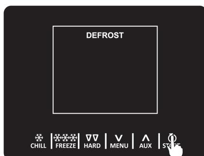
A defrosting cycle can be started manually from the SPECIAL CYCLES menu.
